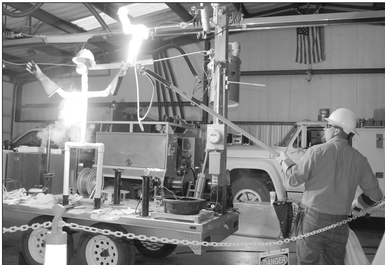
DURING THE MIDWEST demonstration at the fundraiser, Chris Howard uses a piece of rope to conduct electricity from a high voltage wire into a dummy.
