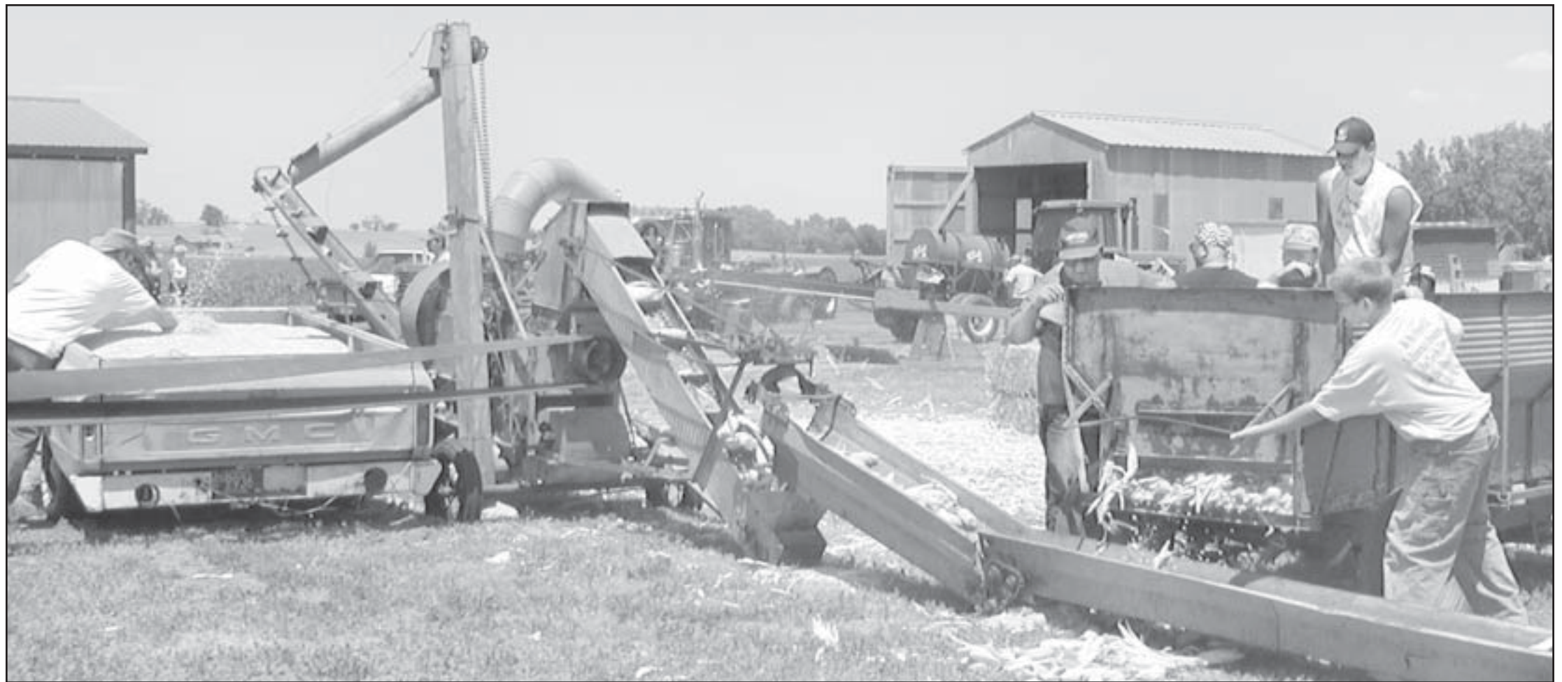
The 1930s era Minneapolis-Moline corn sheller carried ears of corn up a conveyor belt and a steady stream of kernels of corn came out the other end.
