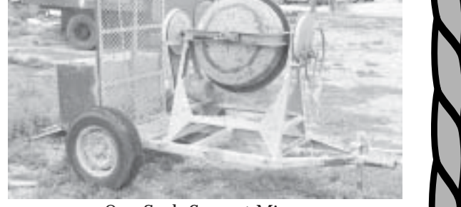
One Sack Cement Mixer
