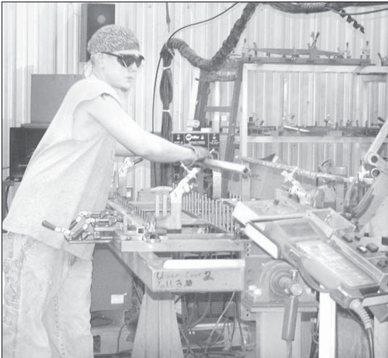
New Age Industrial has 24 welding stations and five precision robots. John Jones (above) loaded pieces of cut aluminum so they can be welded by one of the robots. Mike Wente (below) hung nearly finished racks so they could be finished.
