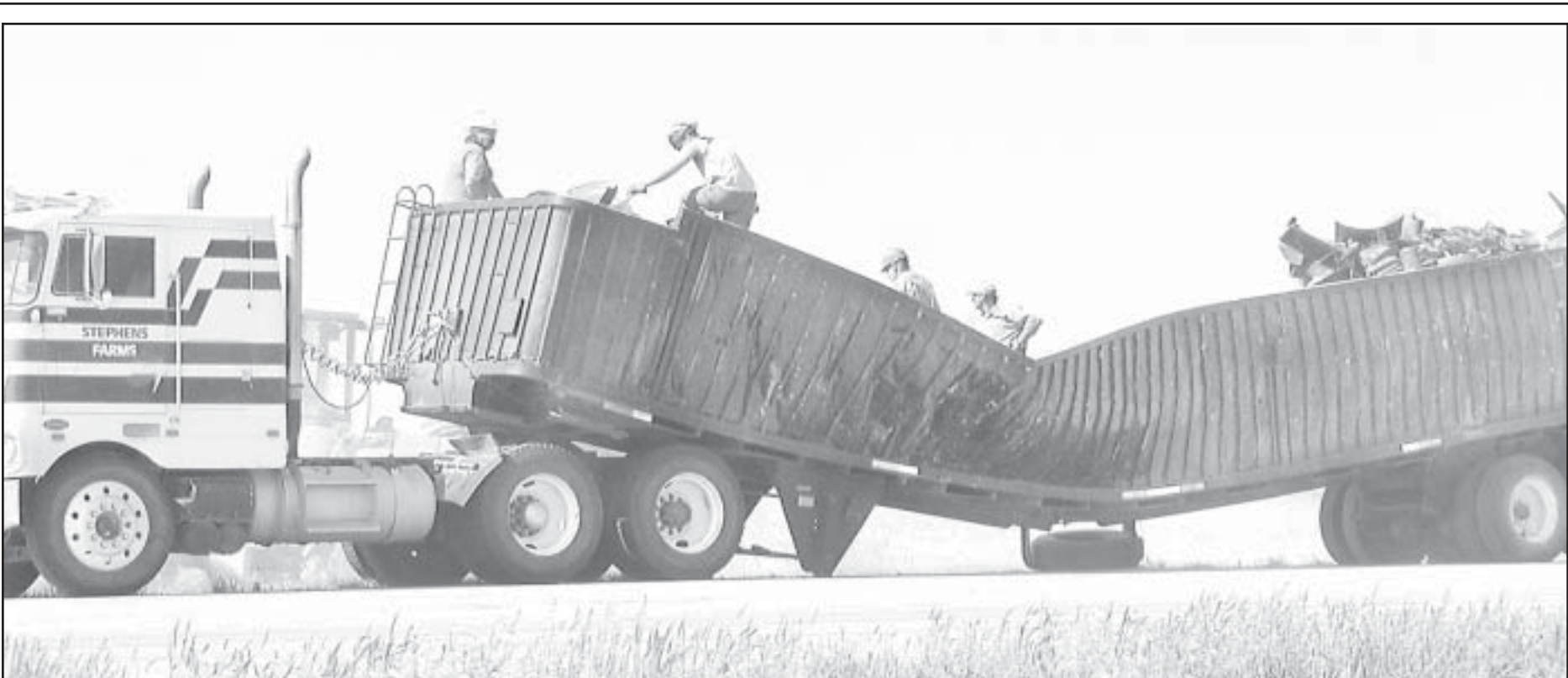
A truck carrying several tons of metal bucketed under its load. Workers from F & F Iron, Norton, unloaded the truck by hand. The accident happened before 8 a.m. Monday, four miles west of Norton on U.S. 36. — Telegram photo by Carolyn Plotts
