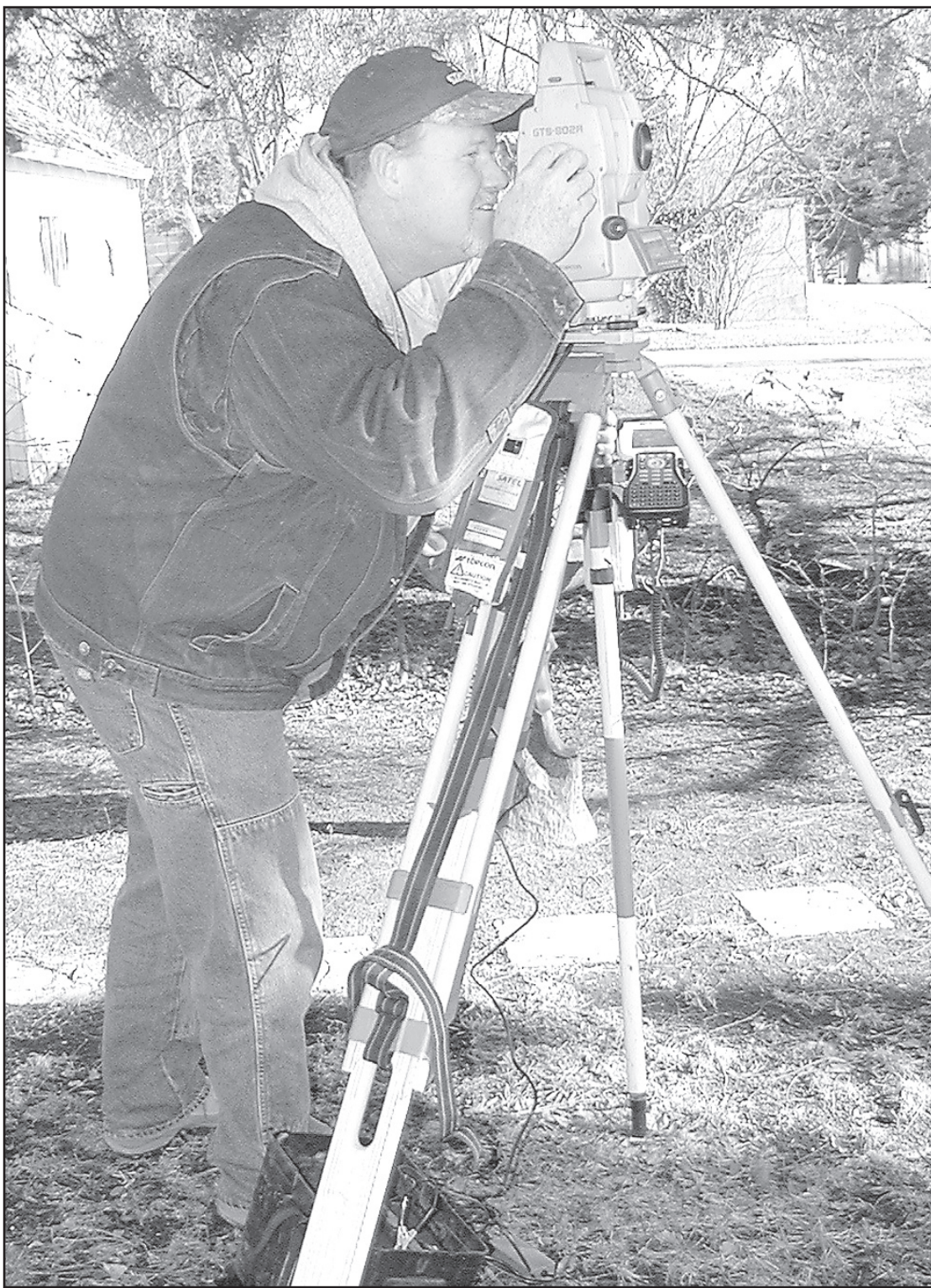
Brian Berlier, BEB and Associates, aligns the tripod of his robotic total station, with laser, that he uses in his surveying business. — Telegram photo by Carolyn Plotts
