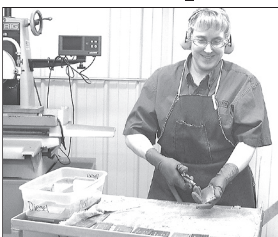
Linda Becker, one of Natoma's 60 employees, is a model for safety procedures. Ms. Becker is wearing protective ear wear, protective glasses, an apron and rubber gloves while she uses air pressure to dry metal parts.
