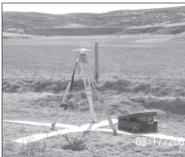
GPSing aerial photo control which leaves white +s on the ground can be seen throughout the county.
