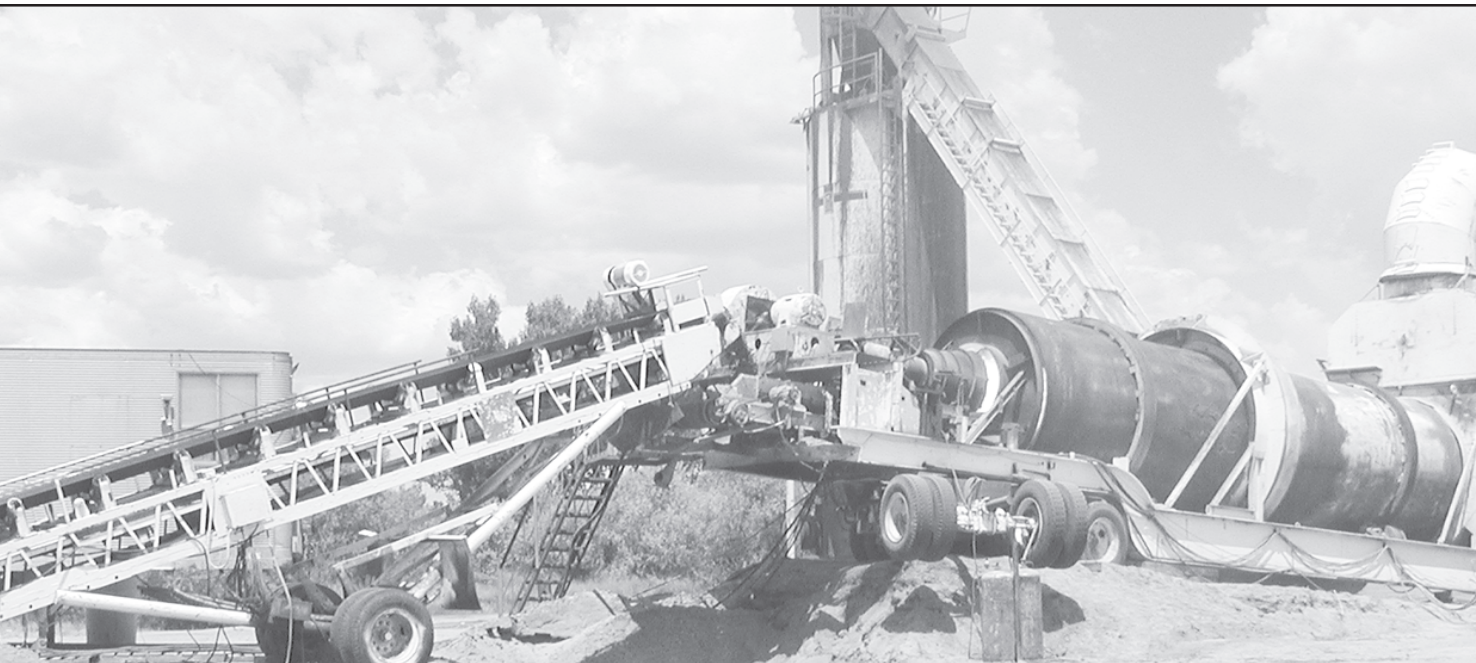
ASPHALT PLANT is set up west of St. Francis. Mix is heated in the huge fire-burning cylinder. Herald staff photo by Karen Krien
