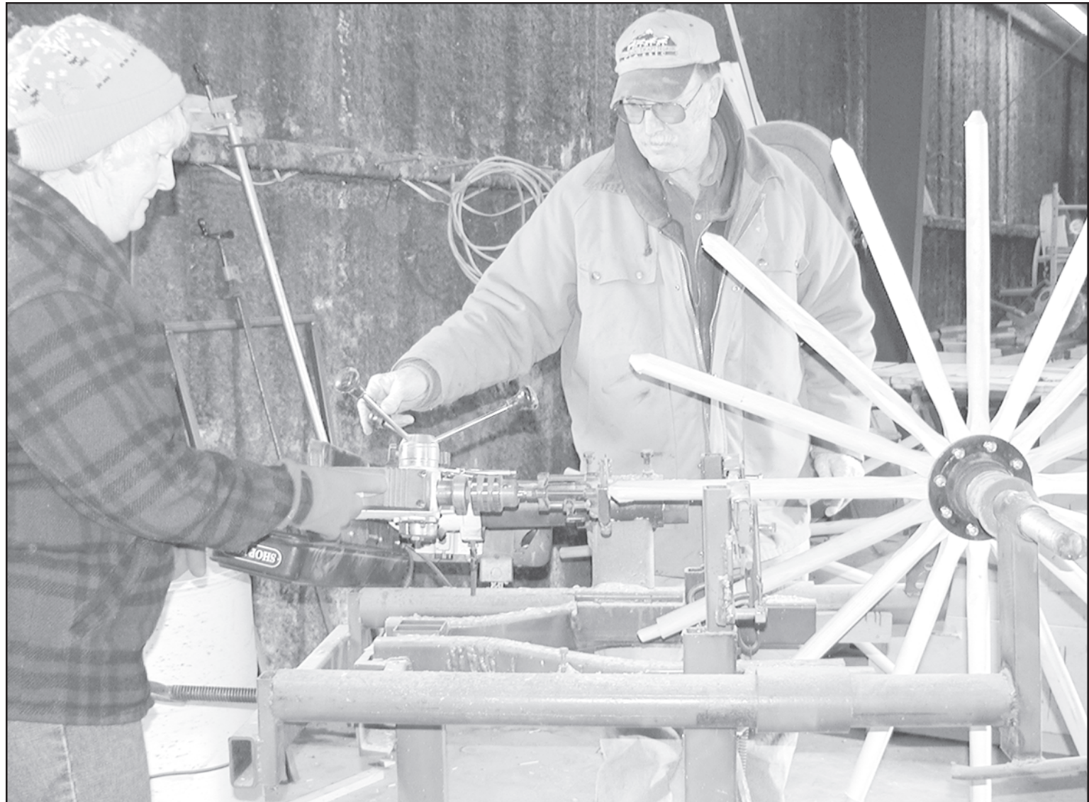
SHAPING THE SPOKES — Dona and Mike McGilvray shape the ends of the spokes with a tennon machine. Some of the equipment is a copy of a machine made before the turn of the century and has an 1870 patent. Herald staff photo by Karen Krien
