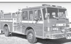
Truck Cummings 6 CTA, 8.3L Diesel, Allison Auto., 500 Gallon Poly Water Tank, 30 Gallon Poly Foam Tank; 1,000 Gallon Per Minute Hale Pump (Certified 2010),
