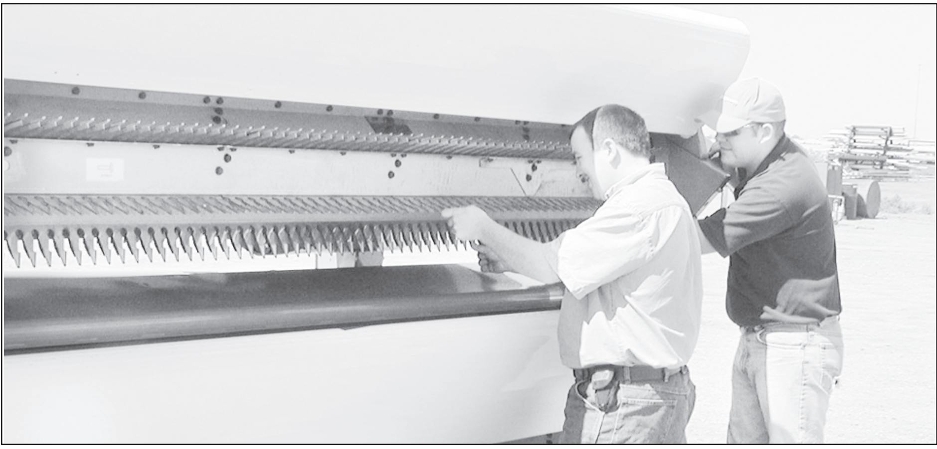
Shelbourne Reynolds General Manager Daniel Morris is assisted by Michael Hawkins, field support, adjusting stripping fingers on the header
