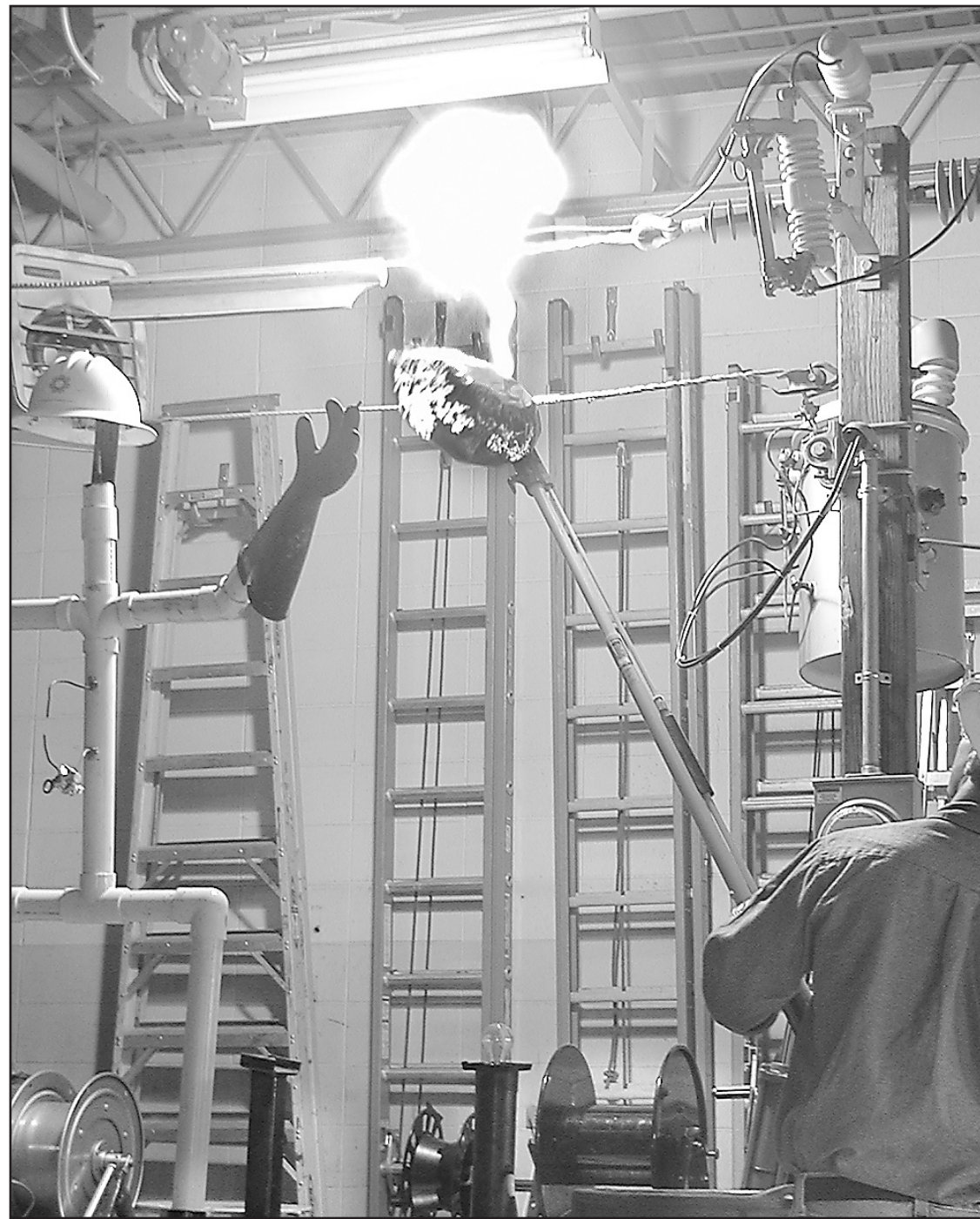
The stick lineman's grapefruit "head" (above) shoots fire when Shane Wentz touches it with a 7,200-volt line. Flying a kite? Here's what happens (right) with a mylar balloon touches an overhead line. The grapefruit represents your brain (below left) and the hot dog your heart on the stick man. At 7,200 volts (below right), the "heart" goes pretty quickly.
