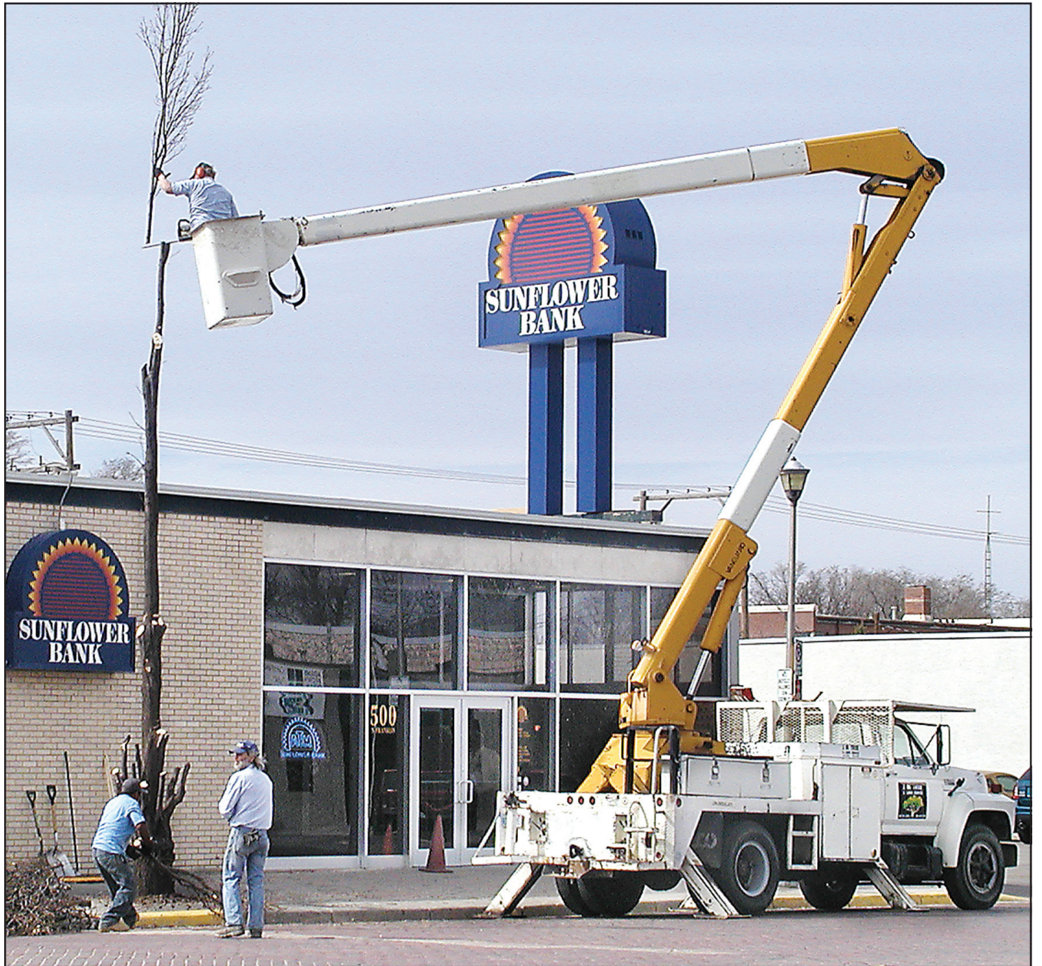
A work crew took advantage of the nice weather Monday to cut down a tree in front of Sunflower Bank. The men cut off each layer of branches going up and then the cut trunk in sections going back down.
