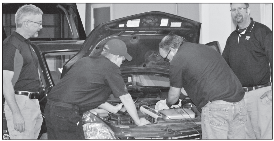
Northwest Kansas Technical College Larry McLemore, collision repair instructor (left), looked on as second year students Roy Williams and Greg Justice made sure the high voltage power was disconnected on this hybrid car. Instructor Curt Goodwin also watched.
