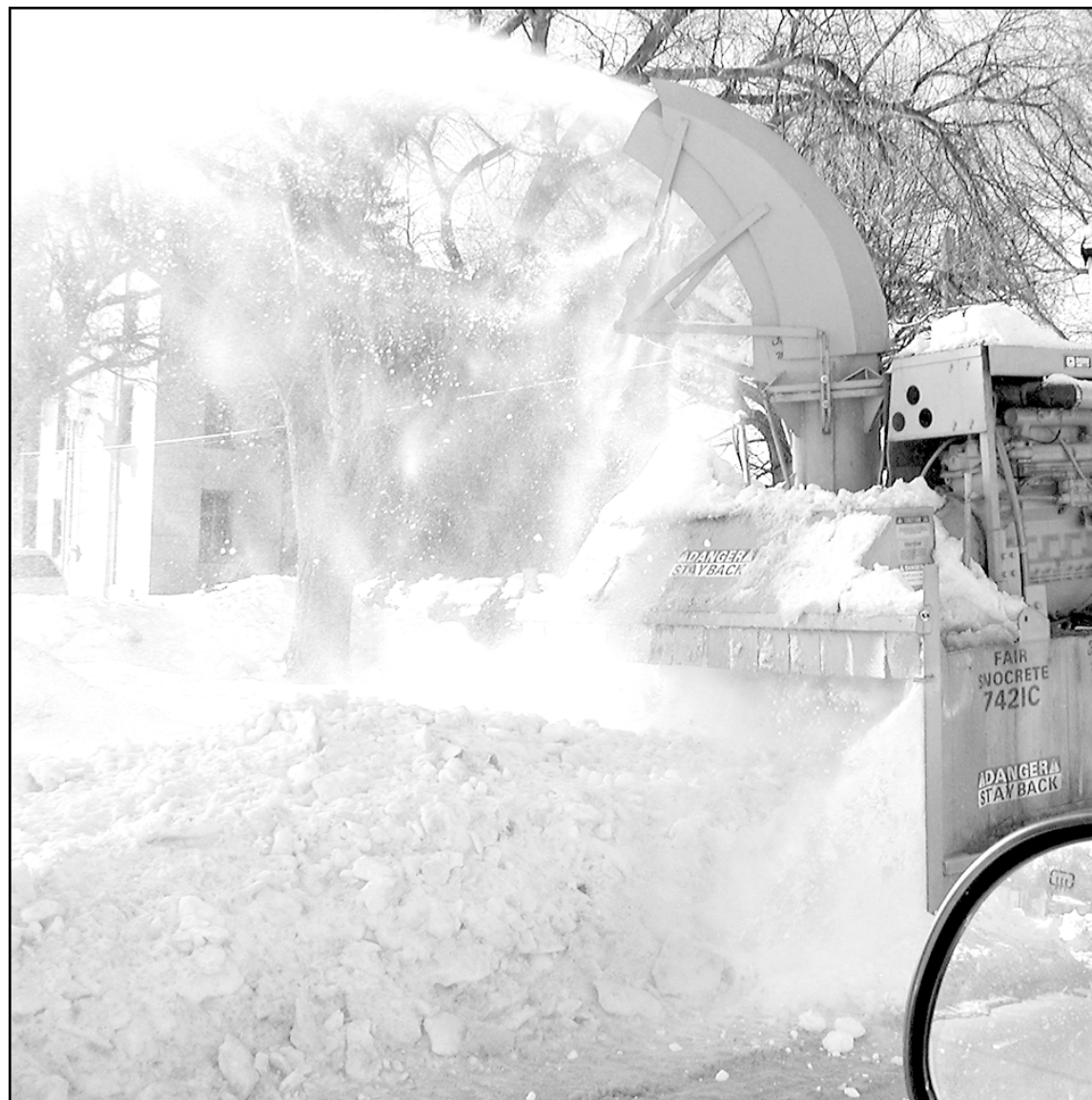
City of Goodland public works crew used a snow blower hooked on a front loader to remove ice and snow from the middle of Eighth Street on Monday morning. Snow removal from the recent winter storms has been a monumental task.
