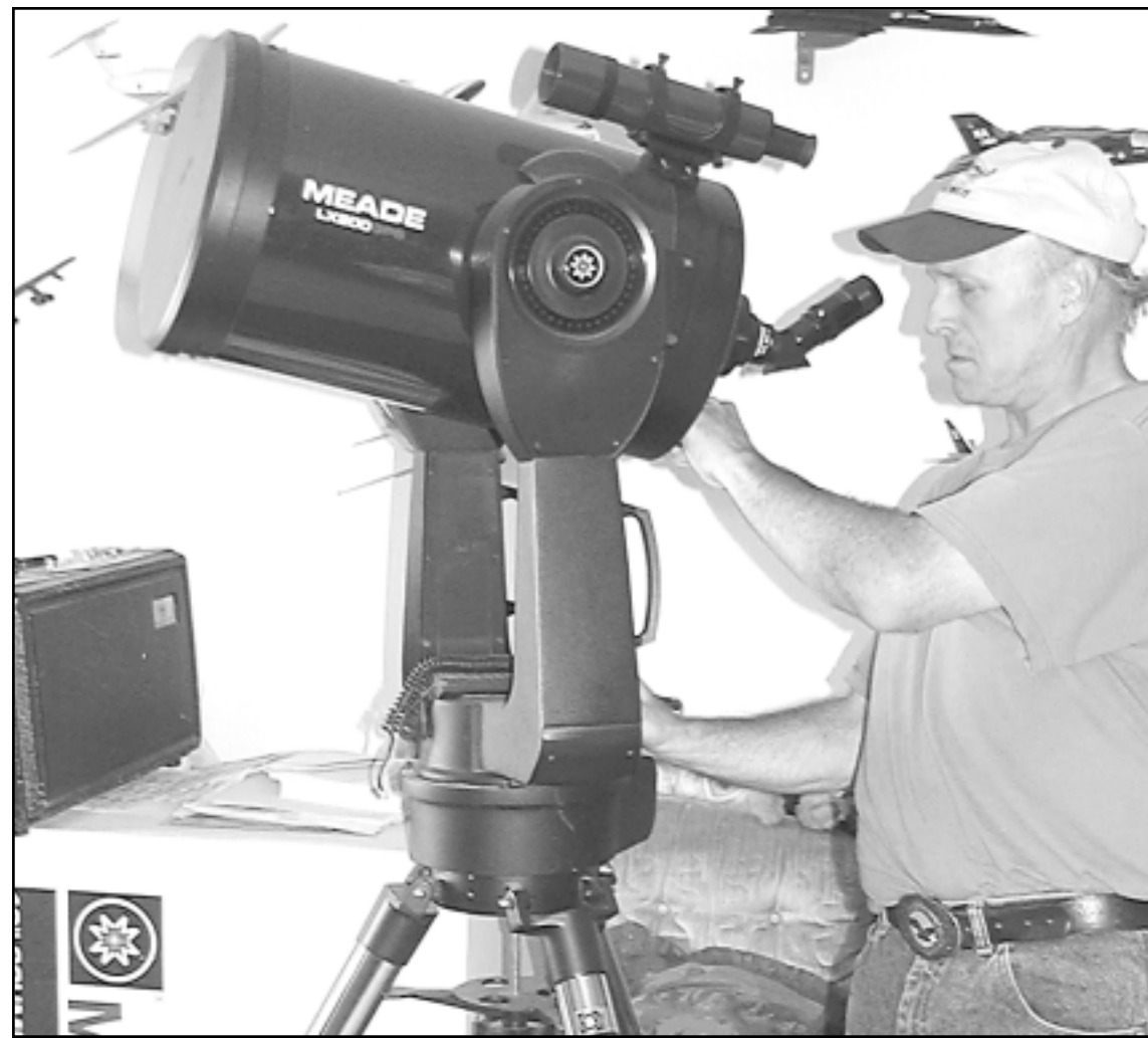
Ron Thompson showed how his telescope can be set to track a star or planet, using a Global Positioning System unit, and how the eyepiece can be used for one person to look through. A camera can be attached to the same eyepiece to take pictures or a video camera can transfer images to a monitor.
