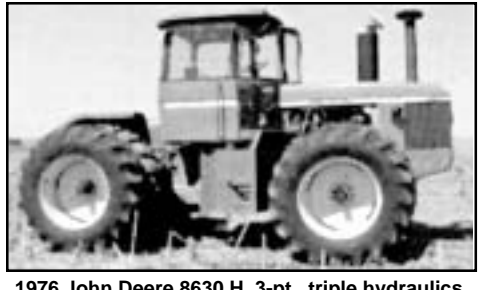
1976 John Deere 8630 H, 3-pt., triple hydraulics, P.T.O., 8350 hrs., S.N.002656R, real good
