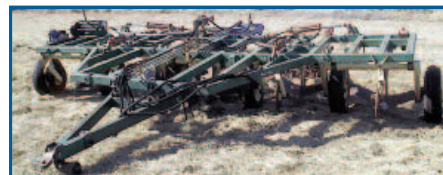
Flex King 5x5 undercutter w/treaders & anhydrous
