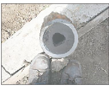
THIS PICTURE OF AN Oberlin water main was taken by Miller and Associates, the engineering firm out of McCook. that's working on the water wells project for the city. The thick stuff around the inside of the pipe is manganese, said Chris Miller, and the reason why the firm proposed building a manganese treatment plant for well No. 11.
