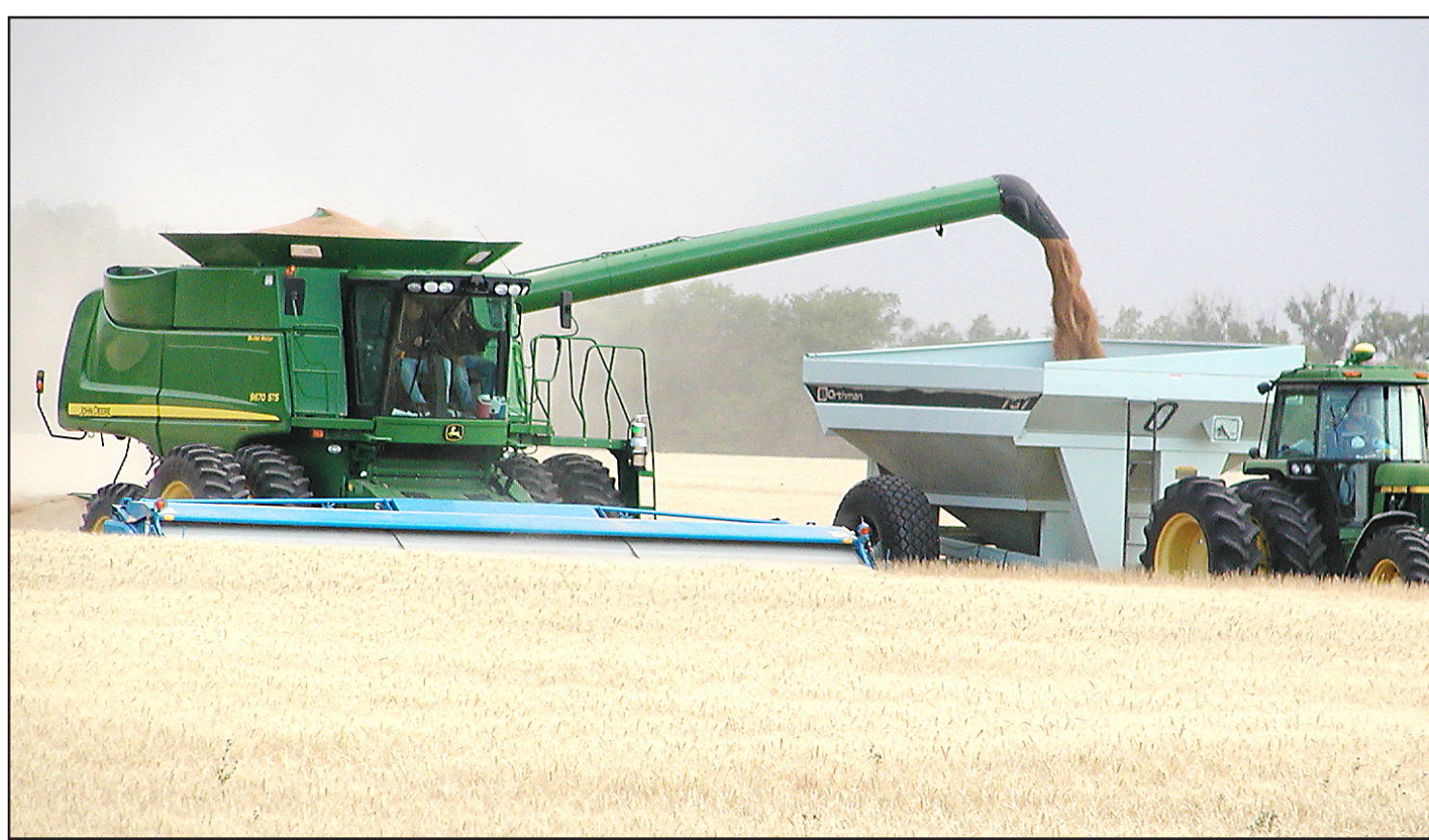
THE JOHN DEERE 9670 STS dumped a load of seed wheat into the grain cart as it rolled through the field, continuing to cut the wheat with a Shelbourne header attachment. — Herald staff photos by Ramell Taylor
